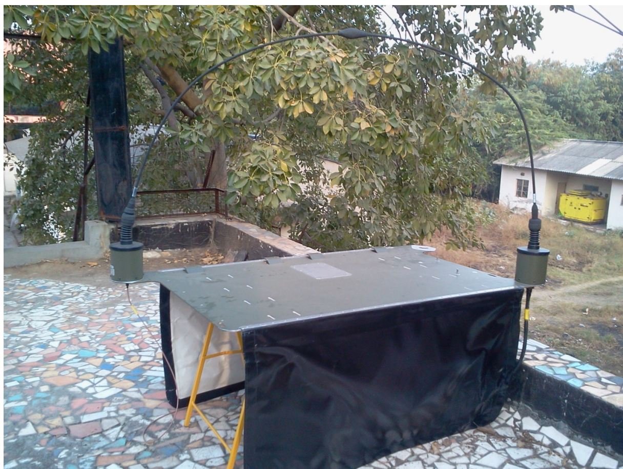
ACTUAL HALF LOOP ANTENNA INSTALLED AT STATIC STATION IN NEW DELHI
